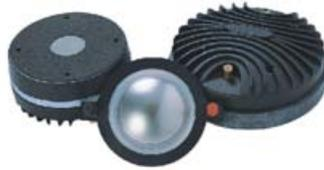
The tweeter adopts titanium diaphragm with high temperature heat treatment, round copper-wrapped-with-aluminum voice coil and compression cavity with linear phase design.
